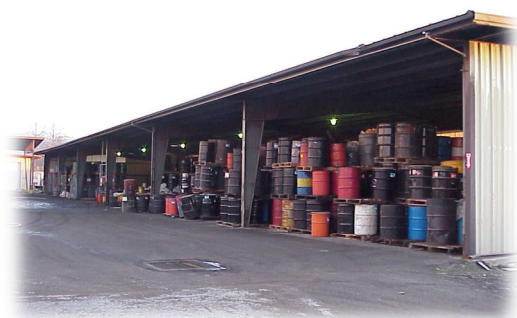
Picture 25. Chemical drums are not stored in a proper way.
